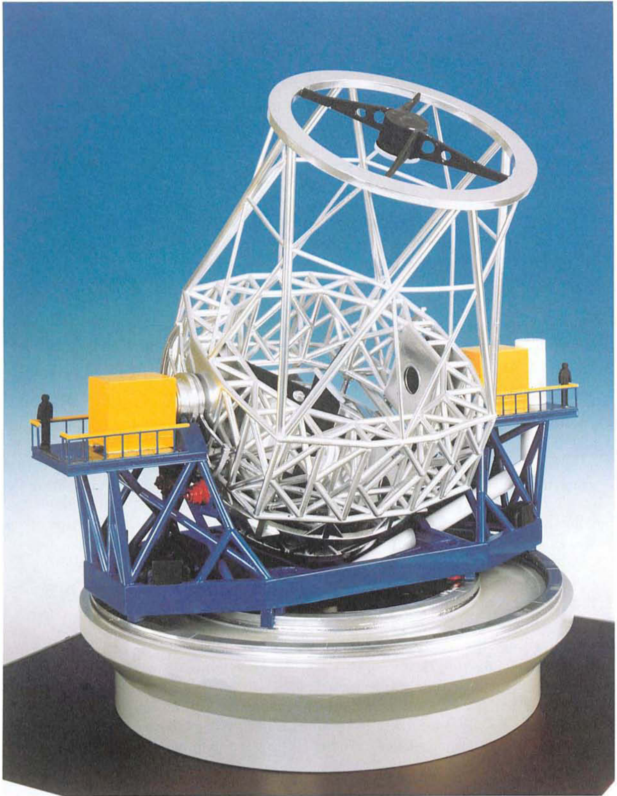
Figure 2.3: Model of the mechanical structure of an 8 metre unit telescope.
